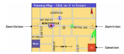
(i) Information - While in Panning Mode, tap the X icon to return to the Map screen. Tap on the North icon displayed to rotate the map so that North or Heading is pointing up.
